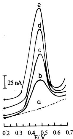
Fig. 5. Adsorptive differential pulse voltammograms obtained after medium exchange for the determination of indapamide in serum samples: (a) blank; (b, c, d and e) serum spiked with increasing concentration of indapamide; (b) 50 ng; (c) 100 ng; (d) 150 ng; and (e) 200 ng per one ml of serum.
