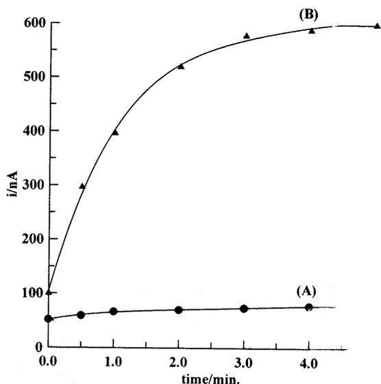
Fig. 3. Effect of accumulation time on peak current for  $5 \times 10^{-7}$  M indapamide at Nj-CPE (A); and Ct-CPE (B); other conditions as in Fig. 2.
