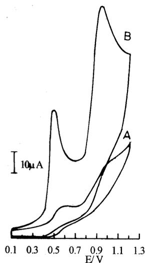
Fig. 1. Cyclic voltammograms for  $2.5 \times 10^{-5}$  Mindapamide in Britton-Robinson buffer pH 4.0; at Nj-CPE (A); and Ct-CPE (B); scan rate:  $50 \text{ mV s}^{-1}$
