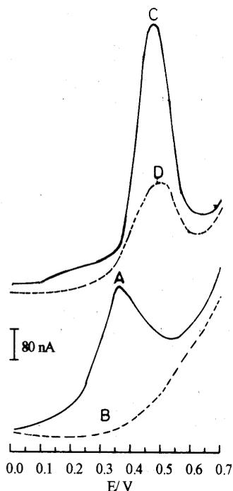
Fig. 4. Linear sweep voltammograms in Britton-Robinson buffer pH 4.0, after 3-min preconcentration at open circuit condition for  $1 \times 10^{-5}$  M ascorbic acid (A and B);  $1 \times 10^{-5}$  M ascorbic acid +  $5 \times 10^{-7}$  M indapamide (C and D). A and C, direct measurement and B and D, medium exchange.
