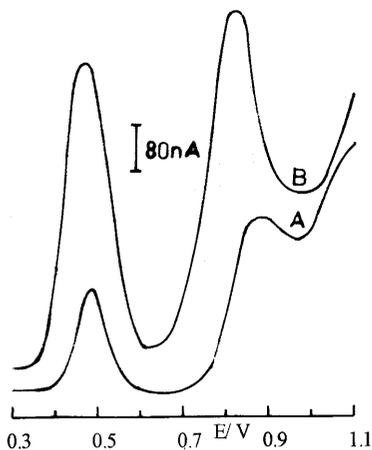
Fig. 2. Differential pulse voltammograms of  $1 \times 10^{-6}$  M indapamide in Britton-Robinson pH 4.0 at Nj-CPE (A); and Ct-CPE (B); scan rate:  $10 \text{ mV s}^{-1}$ ; pulse amplitude 25 mV.
